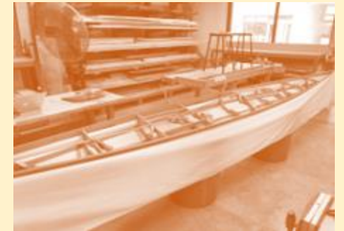
Process Images (Top-to-bottom: Steam bending the coaming, Skinning the frame)
